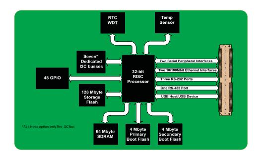
FIGURE 2. VT001 Functional Block Diagram
